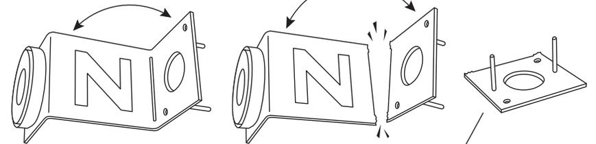
1. Snap the **"Z" bracket** apart by bending.
