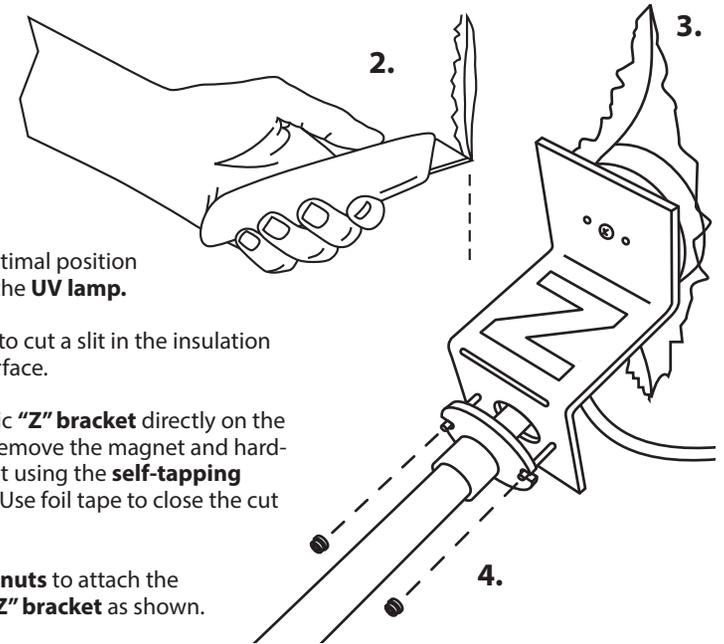
1. Determine the optimal position for placement of the **UV lamp**.
